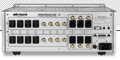
**ABOVE:** A full eight separate line inputs are offered (four balanced on XLRs and four single-ended on RCAs) with duplicate XLR/RCA record outputs and two sets of XLR/RCA preamp outputs. The latter are variable or fixed in 'processor' mode
